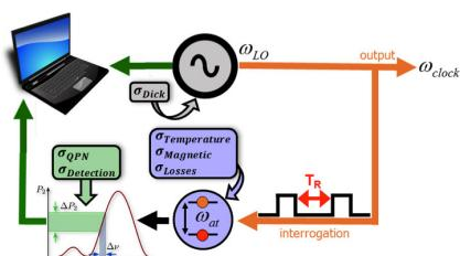
Stability of a trapped-atom clock on a chip,
