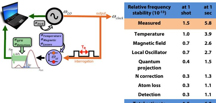
Stability of a trapped-atom clock on a chip,
